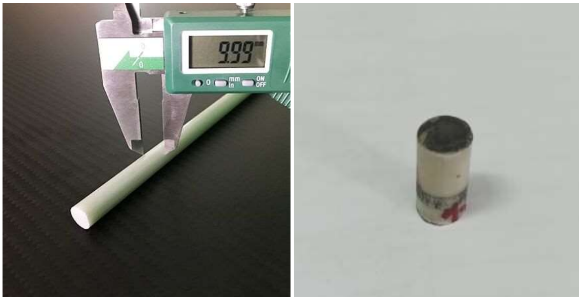
Figure 1. The main material (left) and a wear sample (right)
