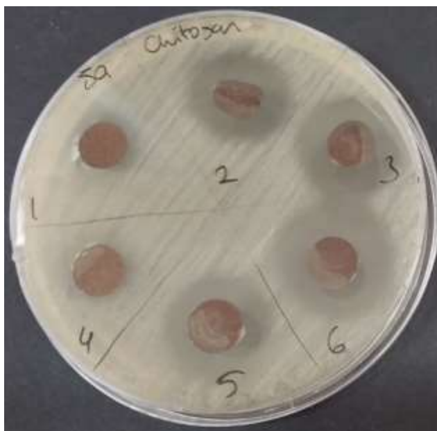
Figure 6: Antibacterial activity of the chitosan films against S. aureus . 1: Chitosan/1.0CL, 2: Chitosan /1.5CL, 3: Chitosan/2.0CL, 4: Chitosan/1.0CL/5.0Chestnut, 5: Chitosan/1.5CL/5.0Chestnut, and 6: Chitosan/2.0CL/5.0Chestnut.
